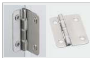
Centre hinge: ▶ Centre hinge 625 is particularly suitable for use with folding doors ▶ Favourable running properties due to abrasion-resistant distance rings with swivel bearing ▶ With fixed steel pin ▶ Steel
