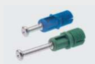
Fast, toolless installation, simply presses by hand into the hole in the carcass side. Easy to tell apart with coloured expanding elements for 8 mm (blue) and 10 mm (green) drill holes.
